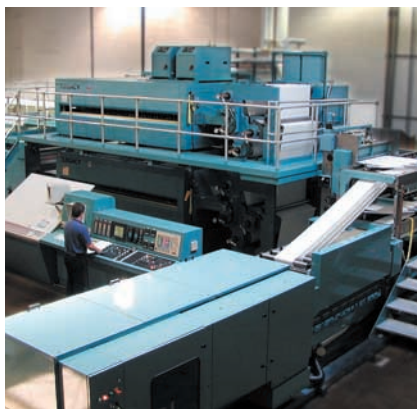
National's newest press is specially made to print high-quality books on lightweight paper.
